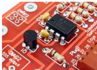
This is what it should look like after Capacitors and Transistors are installed
