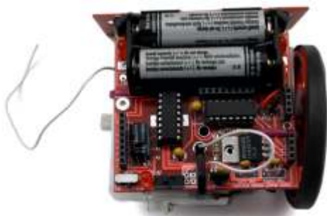
Step 2: Thread wire through to front right side
