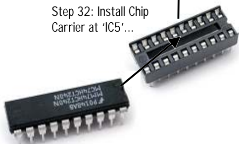
Step 33: ...then install 74HCT240 into chip carrier. Or if you're feeling unlucky, wait until all soldering is done
