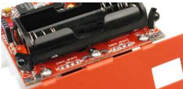
Screwing the plate on with 3 thread-forming screws
