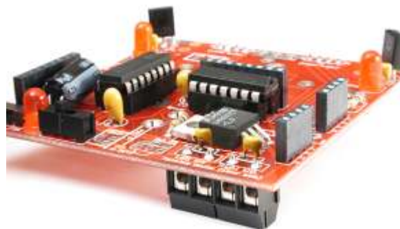
Steps 19: Terminal Blocks Installed
