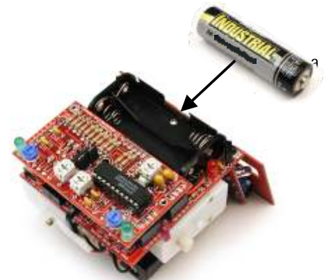
Step 13: Install brainboard Step 14: Install batteries
