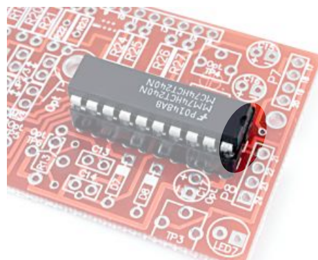
Complete carrier & chip installation. Note the notch position!
