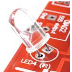
IR LED Installation
