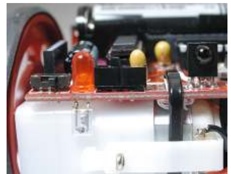
Step 4 (Opt.): Install IR Emitter below LED3
