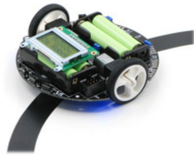
Pololu 3pi robot on a 3/4" black line.
