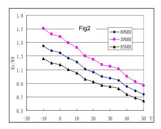
Fig.2 shows the typical temperature and humidity characteristics. Ordinate means resistance ratio of the sensor (Rs/Ro), Rs means resistance of sensor in 100ppm CO under different tem. and humidity. Ro means resistance of the sensor in environment of 100ppm CO, 20°C/65%RH
