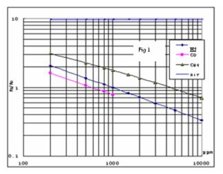
Fig.1 shows the typical sensitivity characteristics of the MQ-7, ordinate means resistance ratio of the sensor (Rs/Ro), abscissa is concentration of gases. Rs means resistance in different gases, Ro means resistance of sensor in 1000ppm Hydrogen. All test are under standard test conditions.
